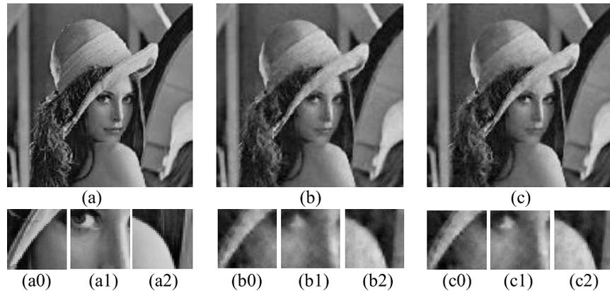
**Fig. 2.** Recovered image Lena ( $256 \times 256$ ). (a): original image; (b): using BCS, PSNR = 28.68 dB; (c): using proposed ABCS, PSNR = 28.90 dB; (a0), (a1), (a2): original image blocks got from (a), cheek, eye and shoulder, respectively; (b0), (b1), (b2): got from (b), PSNR = 25.61, 27.65, 28.81 dB, respectively; (c0), (c1), (c2): got from (c), PSNR = 27.31, 29.90, 31.41 dB, respectively.
